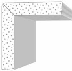
In the first case, cut the two Kerrock elements on the intended joint area under a 45° angle and then glue together. Use an adhesive tape for that purpose.
