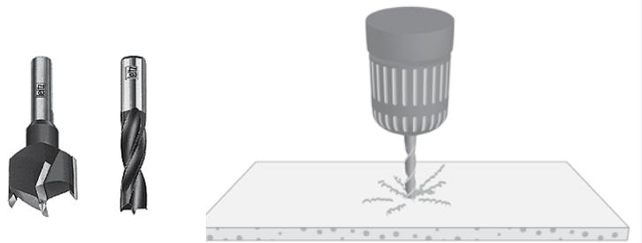
Insert a brass or PVC cork when screwing into the Kerrock surface is required. Make sure the borehole is approx. 10% larger than the screw diameter. Do not forget to insert a rubber or silicone spacer between Kerrock and the second material with joints.
