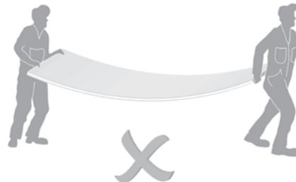
The plates must be transported individually and in vertical position with one hand serving as support and the other for control. It is recommended to use vacuum accessories for transporting heavy loads.
