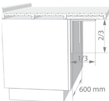
To reinforce the overhang you may also use bearing consoles placed at every 600 mm at least. The vertical elements of the console must be 50% longer than its horizontal part.
