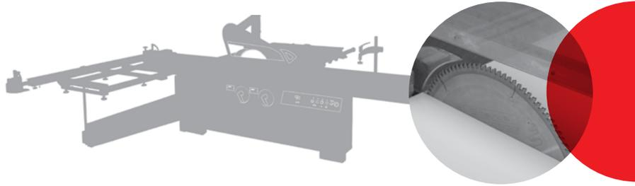
Circular saw blades for Kerrock shall feature both straight and trapezoid-shaped teeth, the latter of which must be 0.3 mm higher than the straight teeth.
