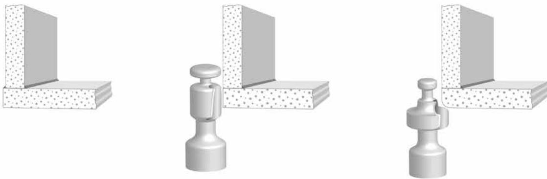
If you opt for the groove, cut a groove into the rear side of the kitchen counter. Its depth should correspond to  $\frac{2}{3}$  of the thickness of the counter, while its width should match the thickness of the element to be glued. Then glue the patch into the grooved part.
