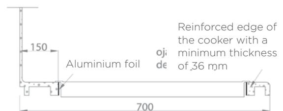
If your work counter is 600 mm wide, you can mount a Kerrock wall cladding; however, it should not be rigidly joined with your countertop. It is to be fixed elastically, as shown in the figure below.
