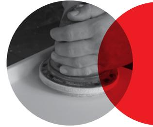
This way you avoid whirls and scratches. Keep the pressure of grinding machine to the surface in limits to avoid overheating of the medium and polymerization of the material which may make the processing more difficult.
