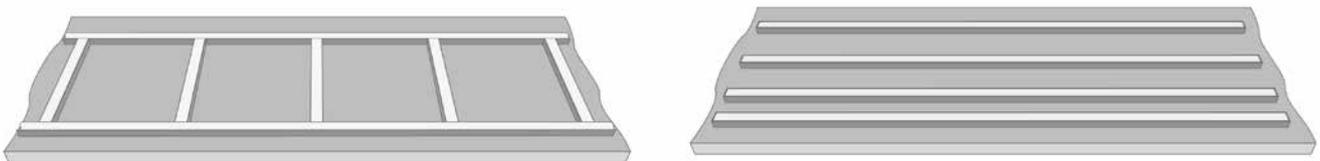
The substructure can also consist of longitudinal reinforcements alone. In this case, fix bearing parts on the front, middle, and rear sides.
