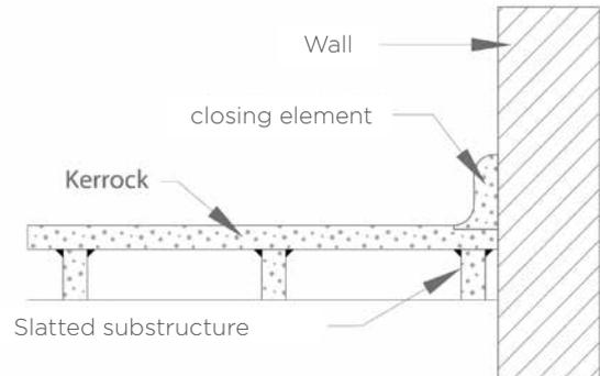
So you avoid troubles related to changes in material due to temperature conditions. The substructure can also be made of wood, wooden plates or metal; note that these must be appropriately protected against moisture. Due to different thermal expansion coefficients, Kerrock plates must be glued to structures from other materials by using permanently elastic glues.
