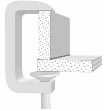
With Kerrock plates containing metal particles (platinum, stardust and graphite), the appearance of the surface and the edge are differing; so make sure the edge is not visible when making joints. There are two ways for doing that:
