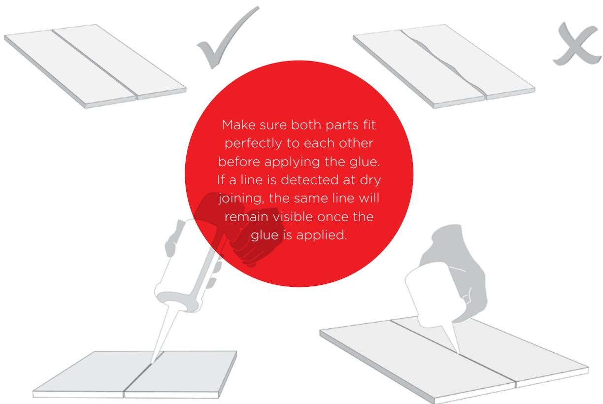
Place the elements to be glued together on a flat surface facing upwards. Leave a 2-3 mm gap between them. Use a template made of material that Kerrock glue does not stick on (e.g. PVC, aluminium, laminated chipboard, waxed or self-adhesive paper, etc.). Insert the glue into the gap between the two Kerrock elements, and then press them together for their final position.
