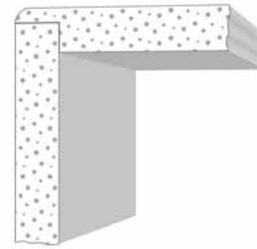
In the second case, cut a groove into the Kerrock plate. Its depth should correspond up to 2/3 of the thickness of the plate, while its width should match the glued element's thickness. Then glue them together.
