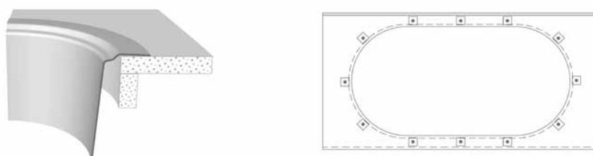
We recommend gluing them tightly along the stainless steel sink to keep their precise location during final installation; this way, the position of your stainless steel sink will simply be defined by the glued hooks.
