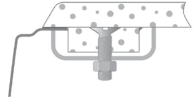
Once the screws are fitted, use the hooks to fix the stainless steel sink. Now you can start processing the finishing edge of the opening. Once the final processing is completed, dismantle the sink and apply silicone glue on its lying surface; fit the sink back in place.
