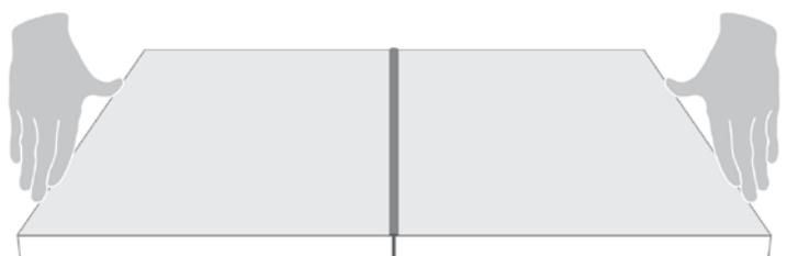
With angle-glued elements, apply the glue on the surface and then press the element perpendicularly to the surface. Use clamps or tongs to fix. We recommend moving the element glued 1-2 mm inside the surface to ensure smooth edging once the process is completed.
