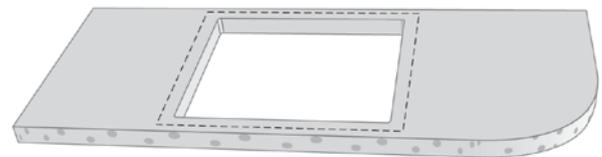
When installing a cooking plate in a Kerrock countertop featuring a Kerrock wall cladding, the distance between them must be at least 150mm.
