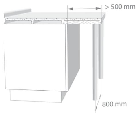
Overhangs of 500 mm or more shall be supported from the ground. Wood or Kerrock material can be used for this purpose. The support shall be placed at every 800 mm.
