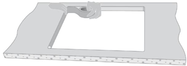
Kerrock is unsuitable for surface-plane-mounted plates.
