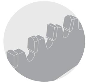
For rougher cuts or for pre-preparation of Kerrock, band saws or jigsaws can be used. Be aware that these may cause tiny cracks in the material, which is why a minimum over-measurement of 5mm shall be taken into account.
