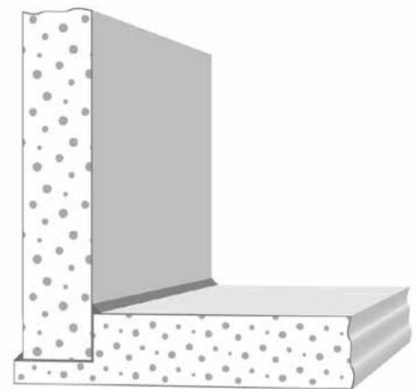
Cut both the glued element and the counter under a 45° angle. Use adhesive tape on the rear side to fix both parts together. Once the glue is applied, fold the glued element to the plate, while the adhesive tape prevents the joint from deformation.
